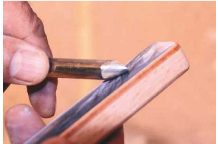
▲ Both the strop and the hone are useful for touching up turning tools
